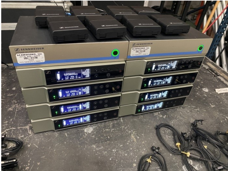
McMullian appreciates the long battery life of the EW-D transmitters which deliver up to 12 hours when used with the lithium-ion battery pack that is available as an accessory (Photo courtesy of Drew McMullian)
